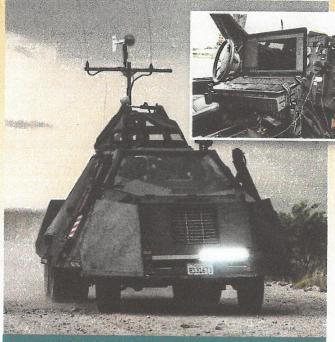
Today, tornado hunters use high-tech gear to follow and study tornadoes. This tricked-out car has armored sides, bulletproof glass, and built-in radar and cameras. If the vehicle is caught in high winds, "tornado spikes" anchor it to the ground. Inside, you'll find sophisticated computers and storm-tracking tools.
